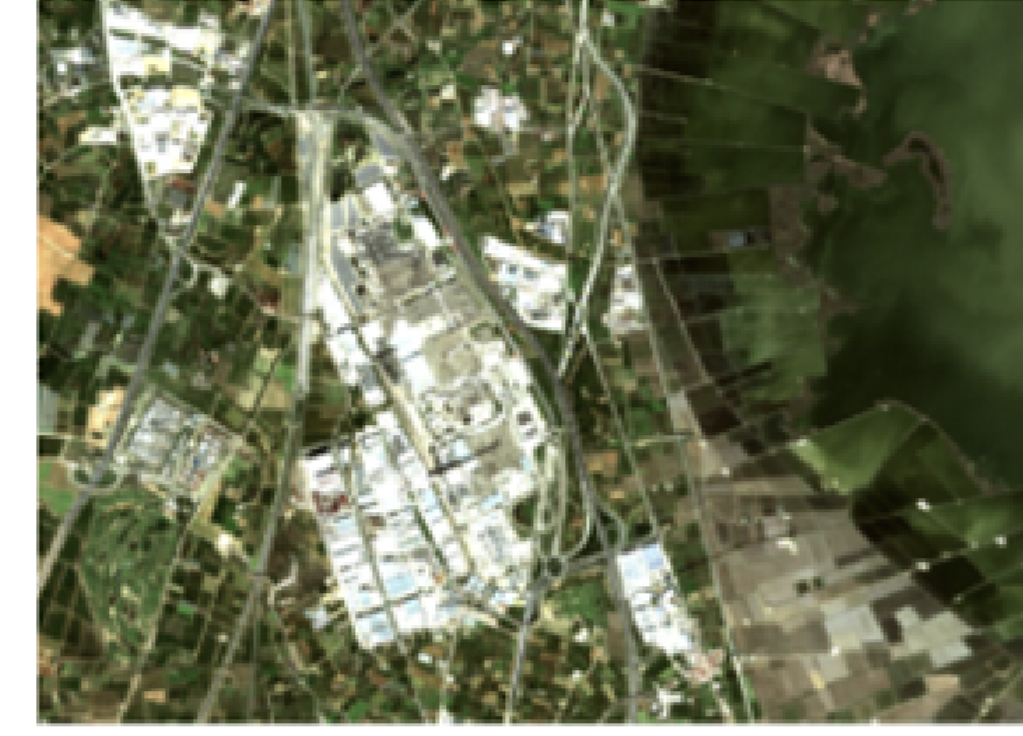
Figure 2: Super-resolved Sentinel-2 image of Ford Plant obtained after applying the deep learning model, showing enhanced spatial detail.
