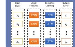
A CNN model with LSTM layers.
